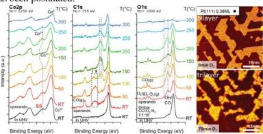
Figure 1: Left AP-XPS of Co2p, C1s & O1s regions, for temperature series from RT to  $300^{\circ}$ C in PROX reaction conditions (6 mbar CO:O<sub>2</sub>:H<sub>2</sub> in a 1:1:10 ratio) of a 0.5ML CoO<sub>x</sub> nanoisland catalyst on Pt(111). Right: STM of the bilayer and trilayer CoO<sub>x</sub> **References**
