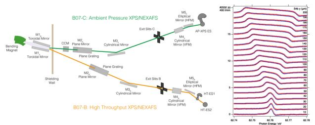
Figure 1. The optical layout of the B07 VerSoX beamlines, and He XAS data as a function of B07-B beamline exit slit opening
