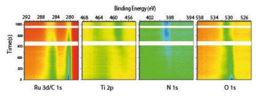
Fig. 1: Time-resolved x-ray photoelectron spectra taken during the first half-cycle of the ALD process.
