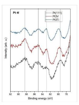
Figure 2. Photoelectron-gas interaction satellite peaks for Pt 4f peak for Pt-based surface
