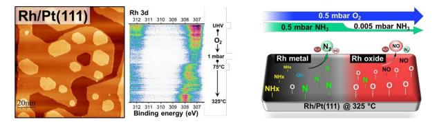
Figure 1. UHV STM (left) and APXPS (middle) demonstrate how surface species (O- and N-) lead to different products during NH3 oxidation (summarized on the right).
