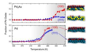
**Figure 1.** *In situ* oxidation of Pd<sub>3</sub>Au (top) and Pd (bottom) surfaces as a function of temperature. The fraction of Pd oxide is deduced from the intensity of the oxide-induced "four-fold surface Pd" peak in Pd 3d<sub>5/2</sub> XP spectra.
