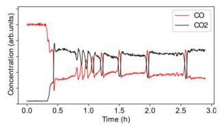
**Figure 1:** CO and  $O_2$  concentrations above a  $Pt_3Sn(111)$  surface.[1] The temperature was ramped up from room temperature to 300°C (reached at about 0.4h) and maintained there. The total pressure was 1mbar and the flow through the reactor 5.5ml/min.
