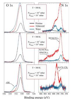
Figure 1 O 1s (left) and N 1s (right core level spectra (hv=650 eV) recorded at different conditions. Black: spectra of the pristine TiO<sub>2</sub> sample, red: after the metal half-cycle, blue: after the water half-cycle.
